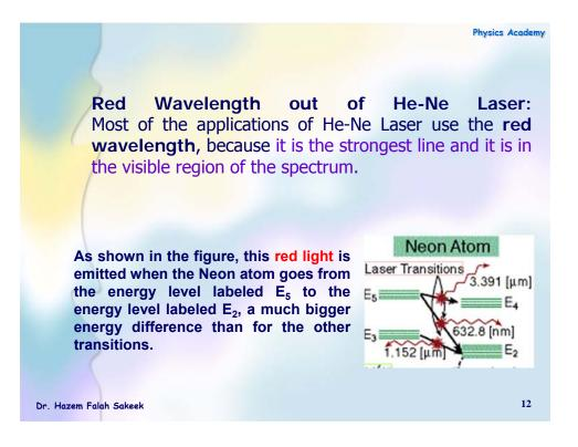
A problem with creating this red light is that a Neon atom in state  $E_5$  may also emit 3.3913 µm radiation. This emission decreases the population of the  $E_5$  level, without producing visible radiation.
